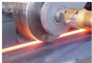
Thermatool's innovative approach to post weld heat treat of HF welded tube and pipe
